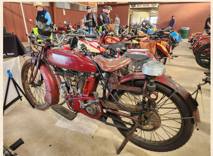
Original 1917 State Police bike. Early memory speedo and friction siren among the original accessories.
