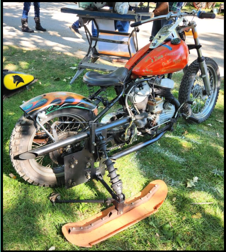
Custom made skis – this bike was raced on the ice in Alaska
