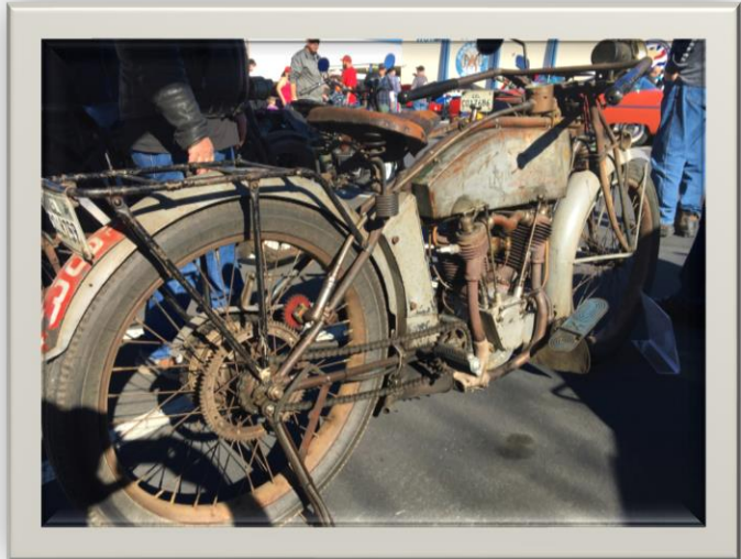
1914 Excelsior Autocycle MODEL 7-T.S. Motor 7 to 10 H.P. Bore 3-21/64" Stroke 3-1/2" Ignition Bosch high tension magnets Carburetor Excelsior-Scheller Model II Transmission Two-speed planetary type Speed Control Right grip-Throttle Left grip-Spark Wheel Base 57 inches
